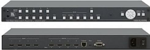
The VSM-4x4HFS is a seamless matrix switcher that can also be used as a 2x2 video wall driver or dual and quad multi-viewers. The unit allows switching between inputs with a clean video cut (frame-to-frame switching with no glitches). The VSM-4x4HFS supports HDMI resolutions with deep color, up to eight channels of audio and includes per-port HDCP and EDID settings
